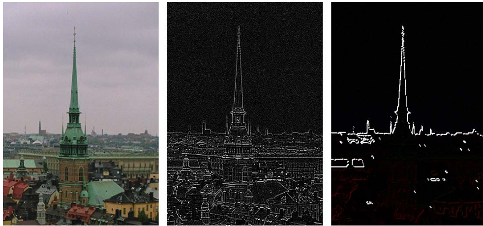
Figure 2: A frame and the processing result after border detection, and after a pipeline of operations.
